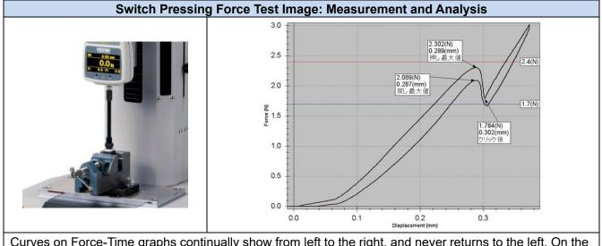
Curves on Force-Time graphs continually show from left to the right, and never returns to the left. On the other hand, curves on the force-displacement graph return back to the left due to base on displacement. The force-displacement analysis helps to provide statistics on hysteresis identification.
