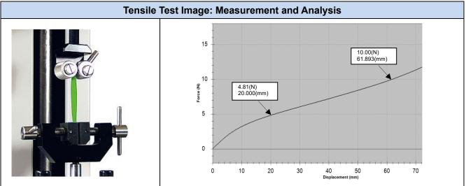
Measuring displacement can help identify relation of the amount of deformation and the force required for the test sample transformation.
