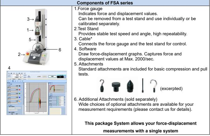
\*FSA-MSL model is for manual operation, hence no cable connections required. Please refer to P3 to check each model.
