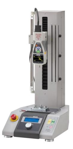
The FSA series is complete test system which can be configured for a wide array of applications requiring both force and displacement measurement. This series draws force-displacement graphs in real time at a high-speed 2000Hz data sampling and it achieves comparing multiple graphs on the screen. The FSA series takes statistical data and contribute to evaluation and analysis.
