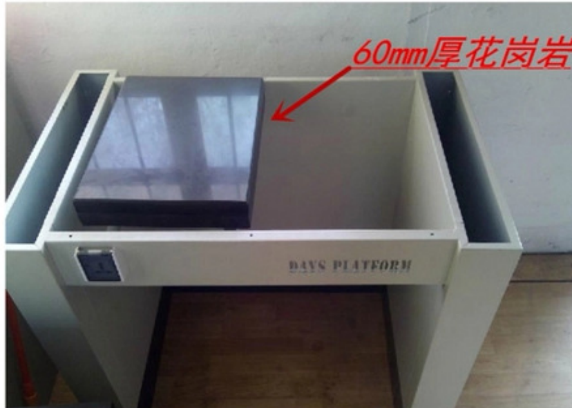
Figure 3.2: 60mm Thickness, Granite Plate – for the particular placing position of Analytical Balances.
