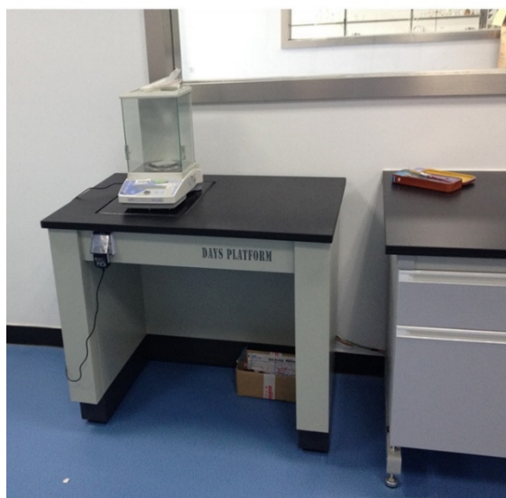
Figure 1.2: Single Analytical Balance Type – Anti Vibration Granite Plate
