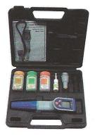
Standard accessories: pH sensor Standard solution pH 4 & 7 Soaking solution Carrying case, instruction manual
