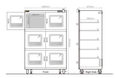
This N2 saving cabinet is designed to control the filling of dry air into the cabinet, so the desired relative humidity in the cabinet can be reached.
