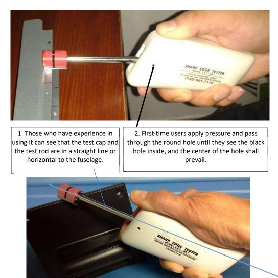
3. The test head with rubber sleeve moves 2 inches (50.8mm) along the tested object, and then returns to the starting point. The total moving distance does not exceed 4 inches (101mm), and the time does not exceed 5 seconds, nor less than 2 seconds.
