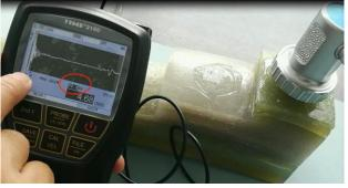
9, Still adjust showing the **MB BLANK**, this function is moving the Gate(small blue triangle) to the signal, while the Gate arrive at the signal, then the thickness value will be calculated and shown by the instrument.
