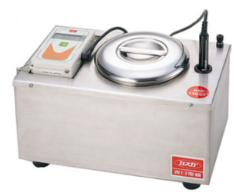
Use of this Faraday cage with the Coulomb meter permits measurement of the amount of electrostatic charge using the Faraday cage method
