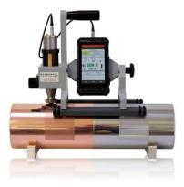
For determination of copper respectively chrome hardness of rotogravure weight have the advantage that they are supposed to be non-destructive as cylinders -simple – fast – accurate. Hardness tests in Vickers range of light the lasting surface indentation is microscopically small.
