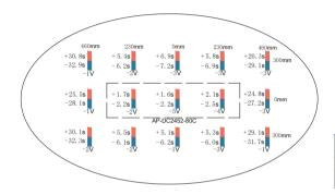
Test standard: ANSI/ESD.STM3.1, SJ/T 11446—2013 Test instrument: Trek 157 static tester Test voltage: ±1000V → ±100V attenuation Test environment: humidity 50±5%; temperature 23±3℃
