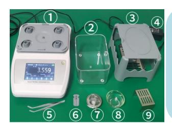
a densimeter, a measuring table, a sink, a power adapter, a tweezers, a calibration weight, an anti-floating frame [the test density is less than the density of water], a set of particle density test components [glass beaker] and stainless steel tennis balls], one instruction manual, and one certificate of conformity
