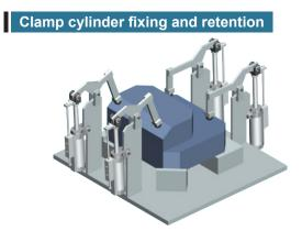
Saves energy because air is not required while locked. (Note that no clamp force operates on the workpiece)
