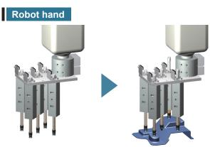
Tracks the workpiece shape simply by pressing the workpiece onto the shaft.
