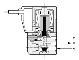
When not energized When the coil is placed in a non-energized state, the plunger will move away from the fixed core and the compressed air will flow from A to R.
