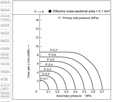
Note) The flow rate will vary depending on the sub-plate, fitting, and tube. Use the values as a reference only.
