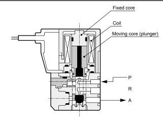
When energized When energizing the coil, the plunger is adsorbed onto the fixed core and the compressed air will flow from P to A.
