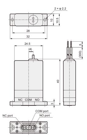
Note: The MR10R-2NC has no hole machined for the NO port. The MR10R-2NO has no hole machined for the NC port. Direct piping
