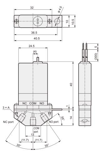
Note: The MR10R-2NC NO port is plugged. The MR10R-2NO NC port is plugged.
