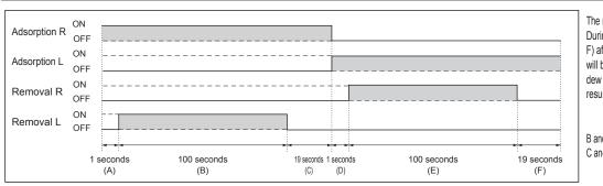
The normal processes are listed on the left. During energy conservation, the state (C, F) after the removal has been completed will be retained. After this, as soon as the dew point degrades, switching will resume to return to the normal processes.
