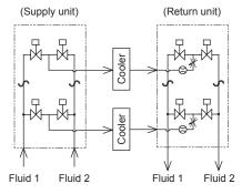
It enables flow of two kinds of fluid (e.g., water and air). Suitable for systems with both coolant and air purge. Each circuit can be controlled separately. (2 units are used)
