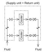
A single unit serves as supply and return units of cooling piping. Each circuit can be controlled separately. Adjust flow rate by using the valve at return side.
