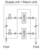
A single unit serves as supply and return for the cooling piping. Each circuit can be controlled separately. Integrated unit for water control One-fluid control
