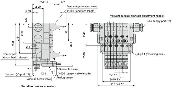
· Negative pressure analog output switch (V□□□)
