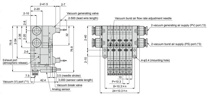
· Negative pressure analog output switch (V \( \subseteq \subsete \))
