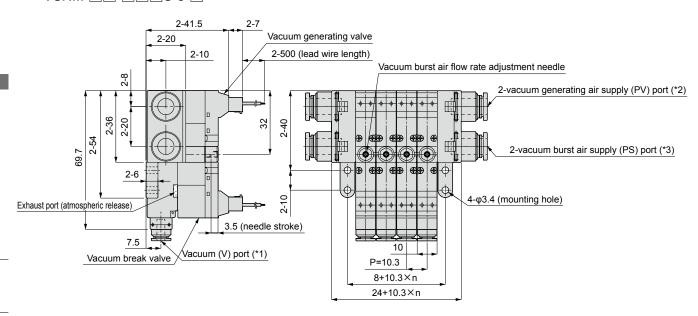
Individual air supply port, with vacuum pressure switch
