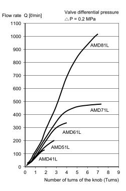
Flow characteristics of the bypass section (water)
