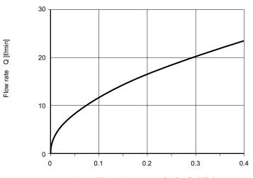
Valve differential pressure  $\triangle P = P1 - P2$  [MPa]
