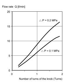
Note 1: Set the adjustment knob at least 1/4 rotation from the fully closed position when using the valve.
