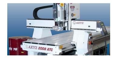
The most compact full-size machine in the AXYZ Series is the 2000. This is perfect for customers with limited workshop space or restricted access. The 2000 Series offers a processing width of 711mm and like all AXYZ Series CNC routers, its configurability enables the 2000 Series to handle the widest range of CNC tooling and application options in the industry.
