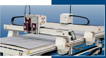
For applications that need a greater vertical clearance such as mould making or three dimensional carving, the standard 150mm gantry height can be extended to 250mm, 300mm or even greater.
