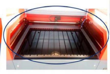
Low power CO2 laser tube is mainly suitable for engraving stamp, for fine carving, laser medical facilities, etc.the laser light spot is small, leaving narrow kurf.
