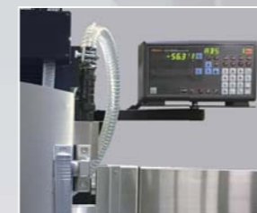
Digital scale for Cross axis display unit built-in operation panel
