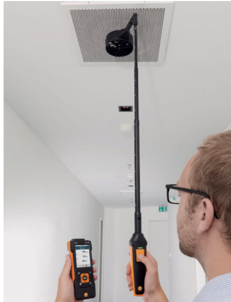
The 100 mm vane probe can be easily combined with the 90° angle and telescope, making measurements at ceiling outlets easier.
