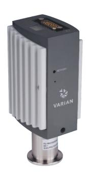
The Varian FRG-720 and FRG-730 combine Varian's Pirani and Bayard-Alpert sensor into a single compact design that provides measuring capability from 5 x  $10^{-10}$  mbar to atmosphere (3.8 x  $10^{-10}$  Torr to atmosphere). Combining these two technologies into a single unit reduces complexity and integration challenges while protecting the Bayard-Alpert sensor from premature burnout.
