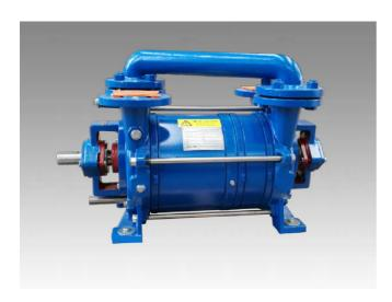
DLV series two stage liquid ring vacuum pump is our new design based on 2SK pumps and combines Germany double-stage pump design criteria. This series has two compression processes, with steady suction speed in high vacuum, or keeping the high vacuum in a wide range of suction speed. Its efficiency in high vacuum is 35%-40% higher than that of single stage pump, but with less energy consumption.
