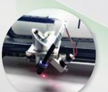
The super user-friendly infrared pointer\* (optional item) helps end users to easily locate the position of objects of any shape vastly eliminating tedious setup time.
