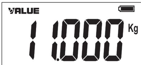
6. If the scale is not connected to the AC power, the solenoid valve will not work. The scale's buzzer will alarm when charging nearly finish (refrigerant  $\leq 0.05$  Kg). when the charge is completed, stop the charge system manually. Press the "Enter" key exit to screen, the scale will display the gross weight of refrigerant tank.
