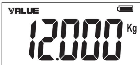
4. Press “Recover” key, the Recovering Indicator will appear, and enter the weight to be recovered, then press “Enter” key. The solenoid valve will open and the refrigerant will start to transfer.
