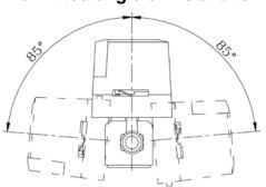
\* Notice: When the valve is mounted on vertical pipe, it must be prevented from dripping. If the valve is used in high-rise building, please install pressure reducing valve on branch pipe of ground floor.
