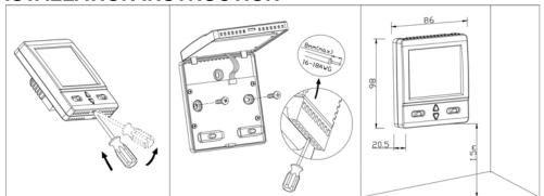
Please remove the wiring terminal from the thermostat before wiring.
