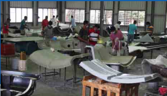
Our own in-house fiberglass reinforce polyester (FRP) manufacturing for better quality control and speedy delivery
