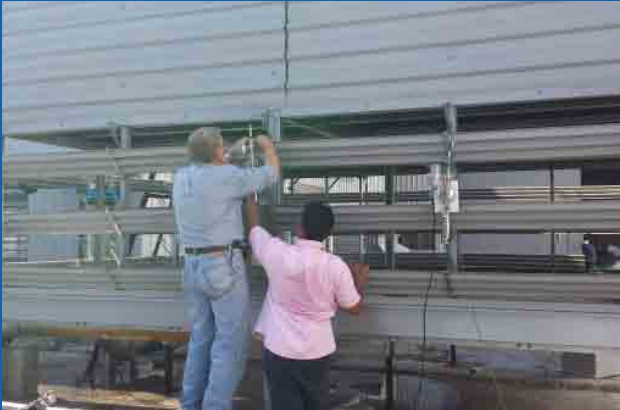
CTI Tester from USA and Genius engineering staff during the setup of measuring equipment for the CTI testing of Genius counterflow tower
