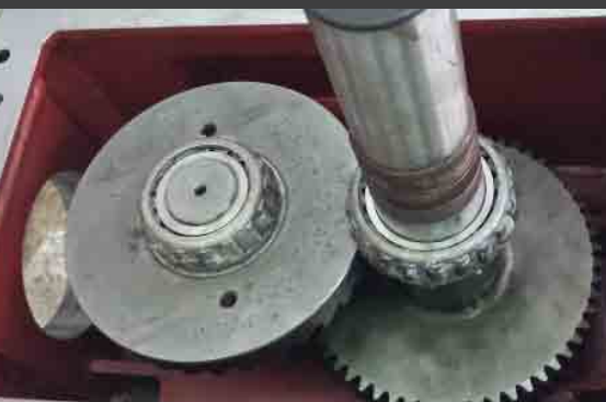
Maintenance and refurbishment of cooling tower gear reducer
