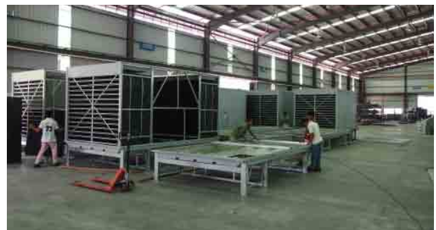
Final assembly for cooling tower
