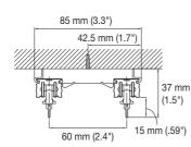
Extra Ceiling Double Bracket Bracket width = 23 mm (.91")
