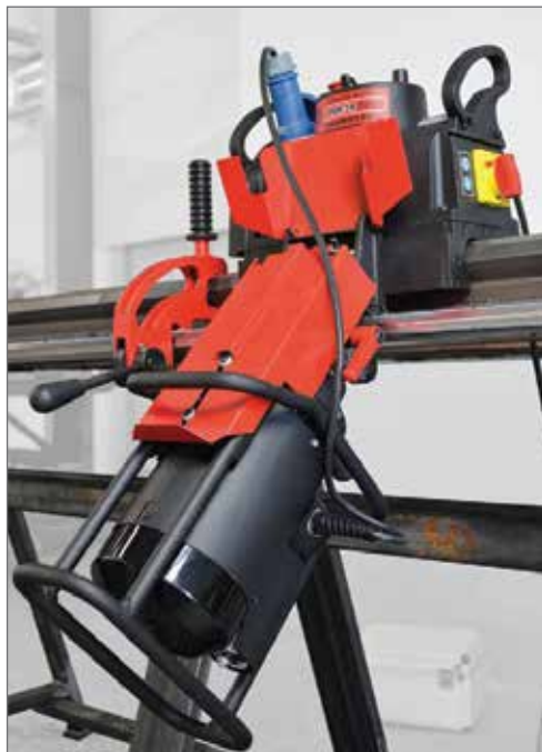
Milling heads for beveling (standard) and for J-groove (option)
