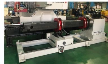
TUBE-250mm*250mm*10mm Cross Dimension and Bevel Cut PIPE-diameter 312mm *10mm Straight and Bevel Cut
