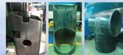
TUBE-250mm*250mm*10mm Cross Dimension and Bevel Cut PIPE-diameter 312mm *10mm Straight and Bevel Cut
