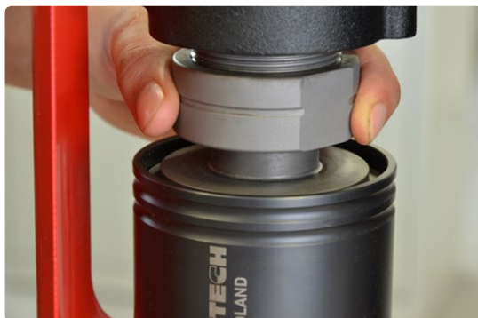
Tapping chuck feat. securing nut
