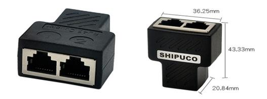
The adapter divide original embedded Ethernet cables (8pins) into two groups (1234/5678). Two groups respectively transmit data with purely physical connection which don't have the function of the assign IP addresses
