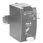
or extends the hold-up time after turn-off of the input power. In times when the power supply provides sufficient voltages, the buffer unit stores energy in integrated electrolytic capacitors. In case of input voltage fault, this energy is released again in a regulated process. One buffer module can deliver 20A additional current.
