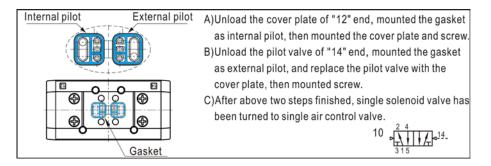
1.3. Double solenoid valve turn to double air control valve
