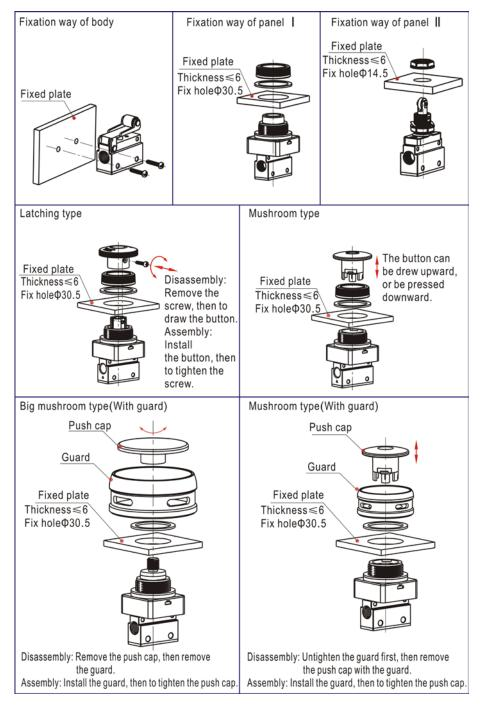
The control set is made of engineering plastic which only allows manual operation and switching valves through metal impact is forbidden.
