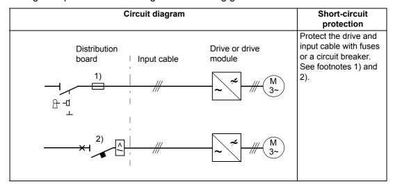
Size the fuses according to instructions given in chapter *Technical data*. The fuses will protect the input cable in short-circuit situations, restrict drive damage and prevent damage to adjoining equipment in case of a short-circuit inside the drive. Circuit breakers which have been tested by ABB with the ACS800 can be used. Fuses must be used
