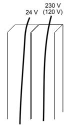
Lead 24 V and 230 V (120 V) control cables in separate ducts inside the cabinet.
