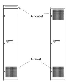
Arrange the cooling air flow through the modules so that the requirements given in chapter *Technical data* are met:
