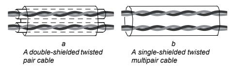
Run analogue and digital signals in separate, shielded cables.
