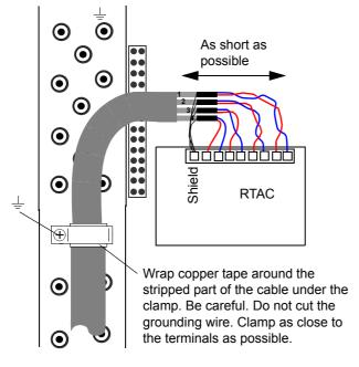
Note 1: If the encoder is of unisolated type, ground the encoder cable at the drive end only. If the encoder is galvanically isolated from the motor shaft and the stator frame, ground the encoder cable shield at the drive and the encoder
