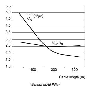
**Note 9:** Sine filters protect the motor insulation system. Therefore, du/dt filter can be replaced with a sine filter. The peak phase-to-phase voltage with the sine filter is approximately  $1.5 \times U_N$ .
