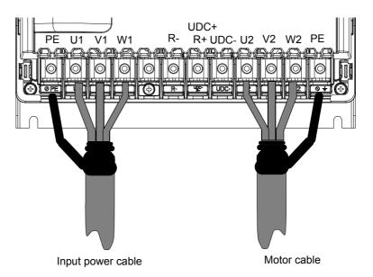
Frame size R6: Cable lug installation [16 to 70 mm<sup>2</sup> (6 to 2/0 AWG) cables]
