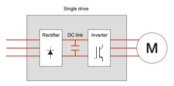
The single drives are complete AC drives that can be installed without any additional cabinet or enclosure. The single drives are available as wall-mounted, free-standing and cabinet-built constructions. The standard protection class of the single drives is UL Type 1 and higher protection classes are available as an option.
