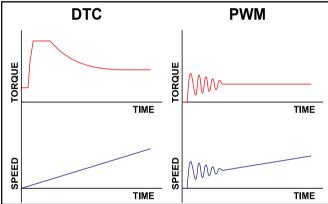
single switching in the drive is determined separately. This feature will always produce the optimal switching combination and can instantly react to dynamic changes such as load shocks or power interruptions. In DTC, there is no need for a separate voltage and frequency controlled pulse width modulator.
