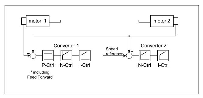
Basically there are several opportunities to realize an *electrical shaft* application. One is shown in the picture. In this configuration converter 2 operates in speed control mode and converter 1 operates in position control mode. That means a position controller is added to the cascade control.
