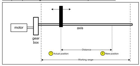
The example shows a component which has to be moved from an absolute position to a new one. The spindle length is fixed what means that the motion is limited.
