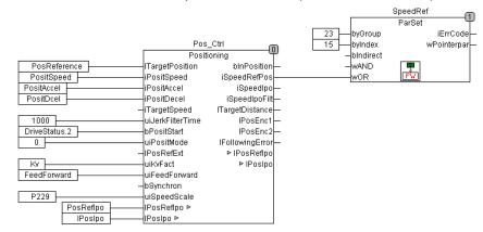
*PosReference* is the main input of function block **Positioning**. The target position has to be connected scaled for 65536 as 1 revolution.
