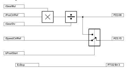
If E-Stop is detected, firmware switches directly to E-Stop ramp
