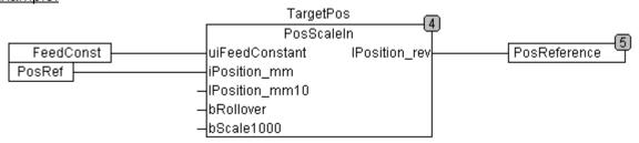
The position reference *PosRef* is the physical distance between point zero and the new point in millimetres. The block calculates by using the feed constant value like the following:
