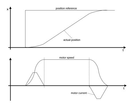
If the software gets a new position the position interpolator starts to calculate the new interpolator reference and the motor drives the component to the new position.
