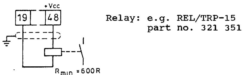
For applications, where the motor must not automatically be without current after having exceeded the maximum cooling temperature of the motor, the resistor R 311 (on soldering posts) must be removed. In case of a controller fault only a fault indication is displayed.
