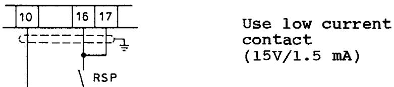
**Caution:** The switch RSP must only be opened at motor standstill.
