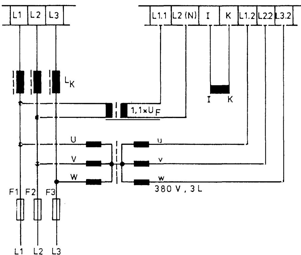
With a mains voltage of less than 380V, the control electronics must be supplied separately or by transformer as shown in the drawing. The wire bridges BR1, BR2, BR3 and BR4 on the boards 4092 or 4093 must be removed.
