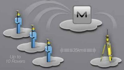
**MAGNET Relay** is a GNSS correction service hosted by MAGNET Enterprise. Subscribers connect a base receiver to the MAGNET Relay service via cellular connection, making the base available for up to 10 rovers.
