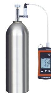
Check with test gas
