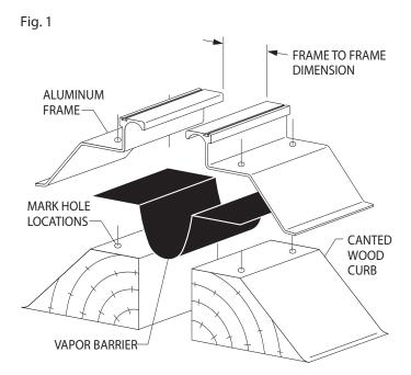
1. Install the architectural joint system on a level surface. To ensure + / - 50% movement, top of canted wood curb must be 1 1/2" (38mm) - 1 3/4" (44mm) wide.
