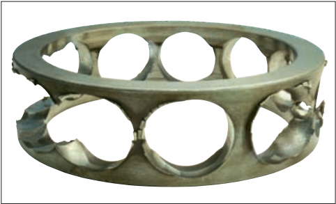
Photo 7-2 Part: Cage of an angular contact ball bearing Symptom: Pocket pillar fractures from a cast iron machined cage Cause: Abnormal load action on cage due to misaligned mounting between inner and outer rings
