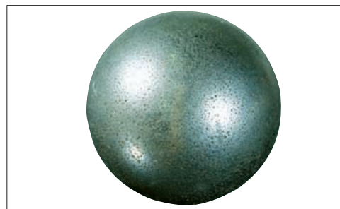
Photo 9-2 Part: Ball of Photo 9-1 Symptom: Pitting occurs on the rolling element surface
