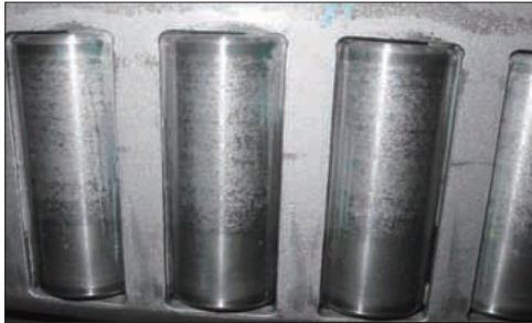
Photo 4-8 Part: Rollers of a large cylindrical roller bearing Symptom: Smearing occurs on rolling surface Cause: Light load and poor lubrication
