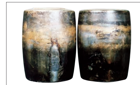
Photo 13-2 Part: Convex rollers of Photo 13-1 Symptom: Discoloration and melting of roller rolling surface, adhesion of worn particles from cage Cause: Insufficient lubrication
