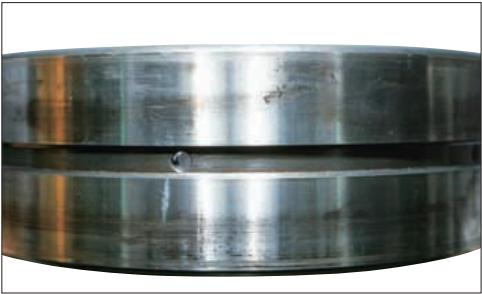
Photo 14-2 Part: Outer ring of a spherical roller bearing Symptom: Creep occurs over entire circumference of outside surface Cause: Loose fit between outer ring and housing
