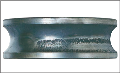
Photo 1-2 Part: Inner ring of an angular contact ball bearing Symptom: Flaking occurs diagonally along raceway Cause: Poor alignment between shaft and housing during mounting
