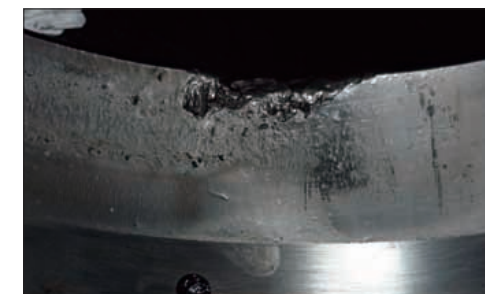
Photo 10-4 Part: Outer ring of a spherical roller bearing (enlargement) Symptom: Example of small flaking and wear combined on the raceway Cause: Insufficient oil film due to poor lubrication leads to wear (primary damage) that progresses to flaking (secondary damage)
