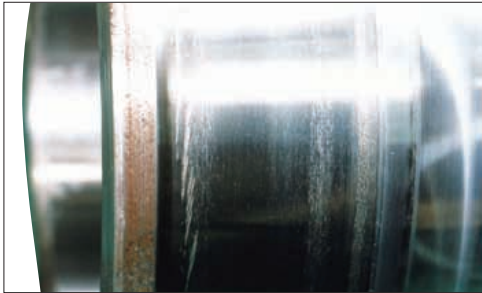
Photo 4-5 Part: Inner ring of a spherical roller bearing Symptom: Partial smearing occurs circumferentially on raceway surface Cause: Poor lubrication
