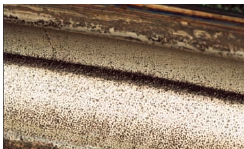
Photo 9-1 Part: Outer ring of a slewing bearing Symptom: Pitting occurs on the raceway surface Cause: Rust at bottoms of indentations
