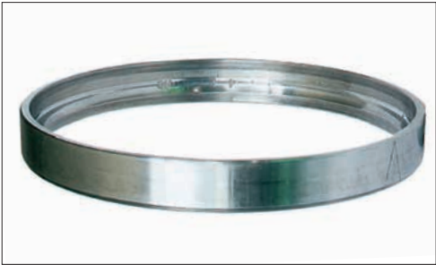
Photo 1-3 Part: Outer ring of Photo 1-4 Symptom: Flaking of raceway surface at ball pitch Cause: Dents due to shock load while stationary
