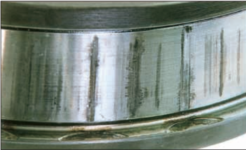
Photo 10-6 Part: Inner ring of a double-row tapered roller bearing Symptom: Fretting wear of raceway and stepped wear on the rib face Cause: Fretting progression due to excessive load while stationary
