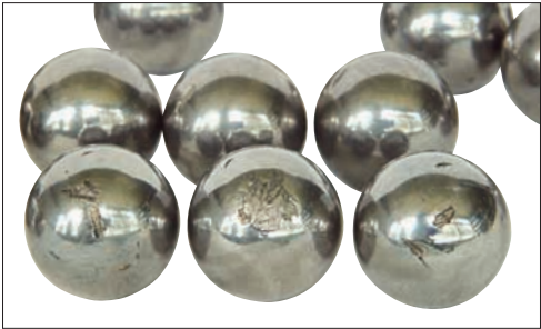
Photo 1-4 Part: Balls of Photo 1-3 Symptom: Flaking of ball surface Cause: Dents due to shock load while stationary
