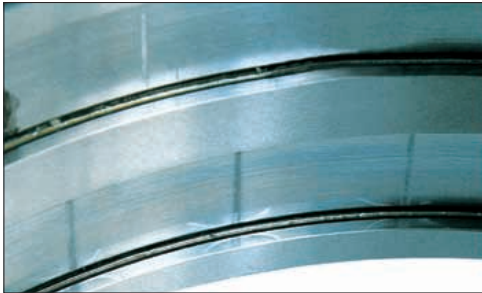
Photo 11-3 Part: Outer ring of a double-row cylindrical roller bearing Symptom: Fretting occurs on the raceway surface at roller pitch intervals
