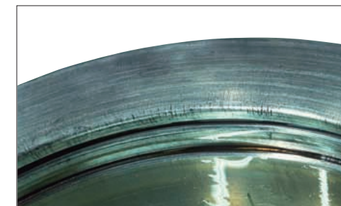
Photo 6-1 Part: Outer ring of a double-row cylindrical roller bearing Symptom: Thermal cracks occur on the outer ring side face Cause: Abnormal heat generation due to contact sliding between mating part and face of outer ring
