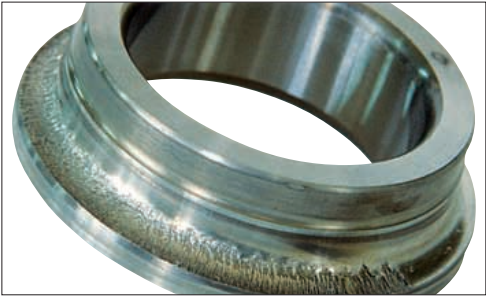
Photo 1-1 Part: Inner ring of an angular contact ball bearing Symptom: Flaking occurs around half of the circumference of the raceway surface Cause: Poor lubrication due to entry of cutting coolant into bearing
