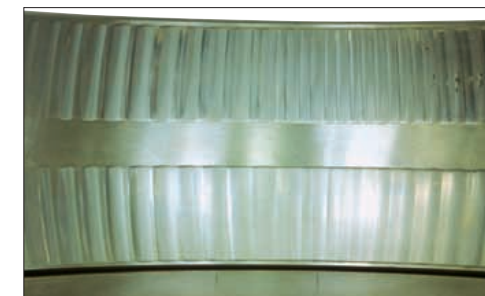
Photo 10-2 Part: Outer ring of a spherical roller bearing Symptom: Wear having a wavy or concave-and-convex texture on loaded side of raceway surface Cause: Entry of debris under repeated vibration while stationary
