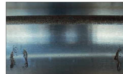
Photo 16-2 Part: Outer ring of a slewing ring Symptom: Rust on raceway surface at ball pitch Cause: Moisture condensation during stationary periods
