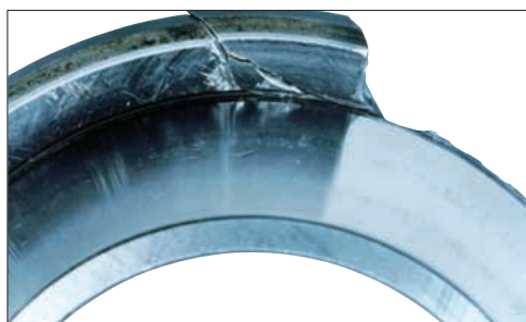
Photo 5-3 Part: Inner ring of a spherical thrust roller bearing Symptom: Fracture occurs at the large rib Cause: Repeated load
