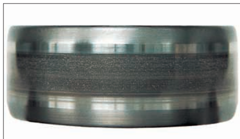
Photo 15-3 Part: Inner ring of a cylindrical roller bearing Symptom: Belt pattern of electrical corrosion accompanied by pits on the raceway surface
