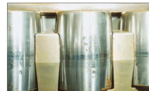
Photo 16-4 Part: Rollers of a spherical roller bearing Symptom: Pit-shaped rust on rolling contact surface. Corroded portions. Cause: Moisture condensation during storage
