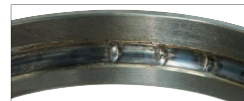
Photo 13-4 Part: Outer ring in Photo 13-3 Symptom: Raceway discoloration, melting occurs at ball pitch intervals Cause: Excessive preload
