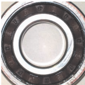
Fig. 6 Internal photo of bearing after test
