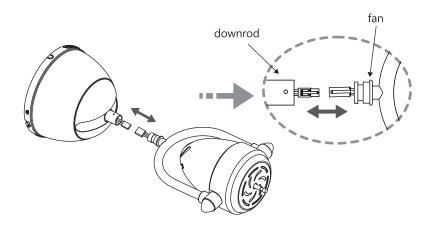
Install downrod and fan body , use hex wrench from screw pack to tighten the 3pcs hex socket screw
