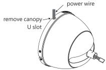
※ According to the power wire connect requirement remove canopy to turn 180 degrees, therefore the U slot can be forward up or down. ■ Connect the plug connector from the downrod to the plug connector from the fan.
