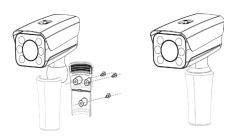
Step 1 Insert the damping ring and waterproof ring of cable into the bracket housing.
