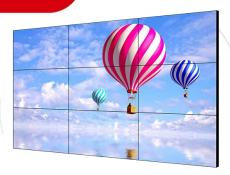
The DS-D2055NH-B LCD display uses an industry-level ultra-narrow bezel design, which enables a bezel width of 3.5 mm between neighboring displays. The adopted direct-lit LED backlighting technology helps achieve ultra-high and uniform brightness of 700 cd/m² without boundary shadows. The display has abundant interfaces for video inputs, such as DVI, VGA, and HDMI.
