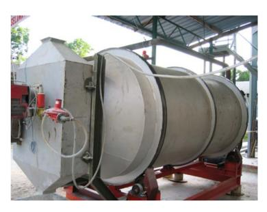
The rotating drum is constructed from mild steel plate and reinforced with trunnion rings. The drum is rotated through a chain and sprocket system driven by a geared motor with guides installed to reduce side movement. The tension of the chain is self adjusting to prevent slipping and irregular movement
